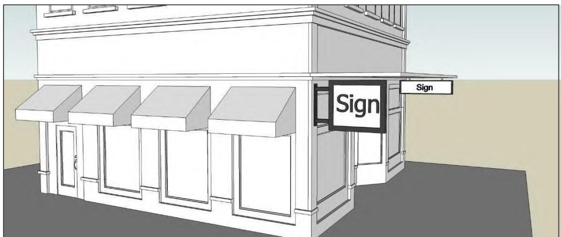
In the above example, both signs have the minimum 8 feet of clearance from sidewalk and are at least 20 feet apart. The projecting sign is 4 ft. X 4 ft. (16 square foot maximum) and the hanging sign is 1.5 ft. high x 6 ft. long (the maximum length to height ratio of 4:1)
