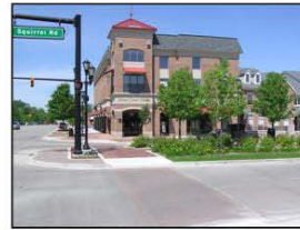
D. Brick pavers along crosswalks
